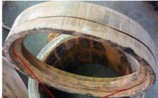
Fatigue crack on on outer ring raceway surface center
